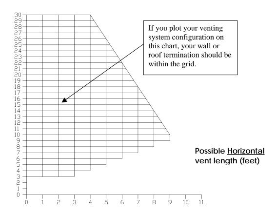
Let's imagine an installation consisting of a horizontal vent coming out at the back of the stove on a total distance of 8 feet. This horizontal run is followed by a Tee and a 6-foot vertical rise. This type installation is not acceptable. As you can see, the vent termination is clearly outside the allowed configuration zone on the chart. The venting system does not have at least one foot of vertical rise for each foot of horizontal run.
